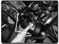
**27.** Install the intake tube into the vehicle and position the tube to the hose and filter.
