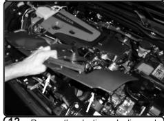
**12.** Remove the plastic push clips and remove the plastic radiator shroud.
