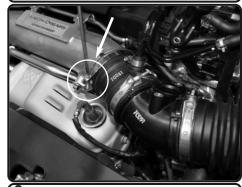
**8.** Loosen the clamp on turbo using phillips screwdriver.
