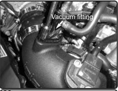
**28.** Install the vacuum fitting to the intake tube using the 2 original screws from step 7. Secure and tighten.
