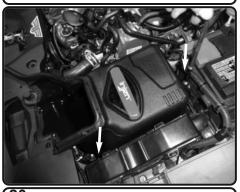
**20.** Once seated properly use the OEM screws from step 6, and secure the air box.
