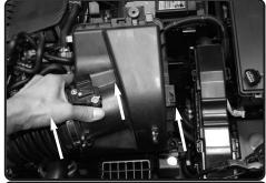
**10.** Lift up and remove the airbox.
