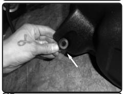
**17.** Remove the 2 smaller OEM grommets with crush washer from the OEM air box and install to the mounting points on injen EVO box.
