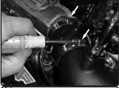
**31.** Adjust intake tube for proper fitment, secure and tighten all clamps.
