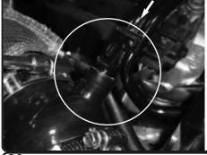
**30.** Install the crank case hardline from step 9 to the step hump hose.
