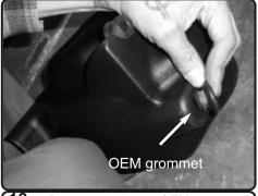
**18.** Remove the larger OEM grommet and install to the hole on the bottom of the air box.
