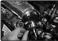
**24.** Install the step hump hose with clamps provided to the throttle body and position. Do not tighten.
