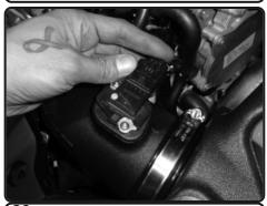
**29.** Re-connect the MAF sensor harness. Secure and tighten.
