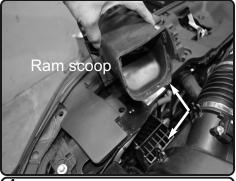
**4.** Now lift up and pull back the Rubber ram scoop. Note: there are plastic fittings holding in scoop, pull rubber away from fittings.
