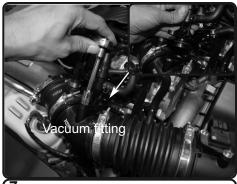
**7.** With 10mm socket, remove the 2 screws holding in vacuum fitting. Carefully pull back fitting.
