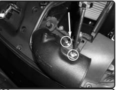
**26.** Now install to the new injen intake tube and secure using original screws. Secure and tighten.
