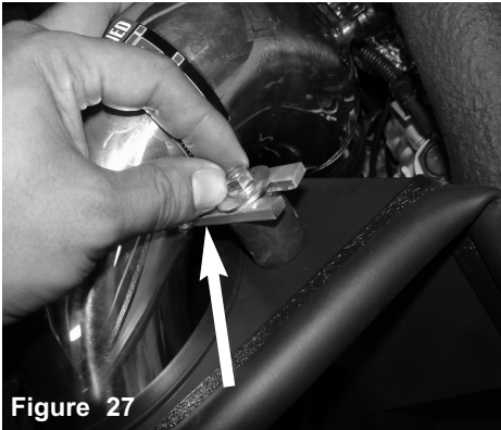
Figure 27 Secure the bracket using fender washer and M6 nut.
