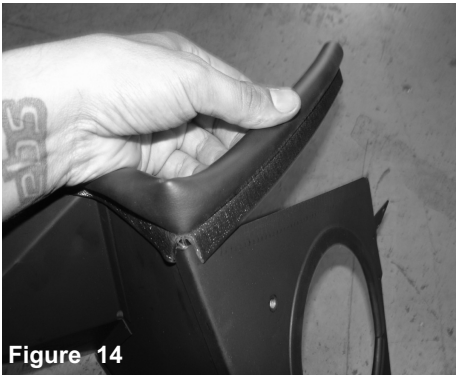
Figure 14 Attach the rubber trim to the top of the heat shield. You can cut a notch into the corner if necessary for easier installation.
