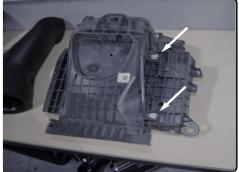
**15.** Remove the screws and remove the lower part of the battery box.
