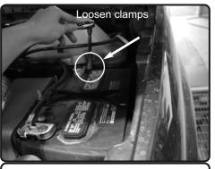
**2.** Loosen the negative terminals on both batteries.
