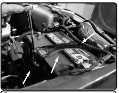
**8.** Remove the battery from the passenger side only and remove from vehicle.
