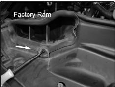
**10.** Remove the push clip from the factory ram scoop.
