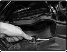
**20.** Install the rubber inlet duct and secure using OEM clip.
