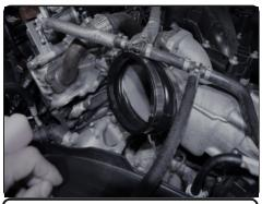
**29.** Install the hump hose to the turbo inlet. Only tighten the clamp on the turbo side for now
