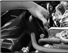
**24.** Install the air filter into the air box and rotate a 1/4" turn until filter locks and seats into position.
