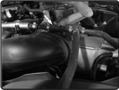
**3.** Loosen the clamp on the intake tube using 7mm nut driver. Pull back the coolant line from the intake tube.
