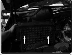
**7.** Now lift up and remove the air box out of the vehicle.
