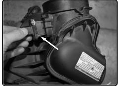
**28.** Remove the 2 screws and remove the MAF sensor.
