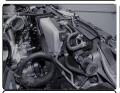
**23.** Push the A/C line towards the coolant reservoir to create clearance for the filter and tube.
