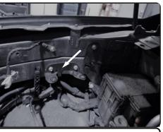
**14.** Remove the OEM air box bracket out of vehicle.
