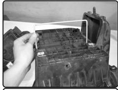
**16.** Remove the battery tie down. This will be reused in the Injen kit
