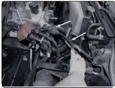
**20.** Remove the electrical tape holding the cable indicated by the arrows from the power cable. Then use electrical tape to tape all exposed wires. This will allow the power cable to extend to the new battery location.
