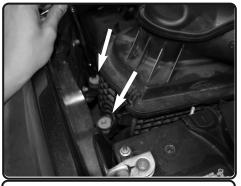
**4.** Remove the 2 bolts holding in the bottom of the air box.
