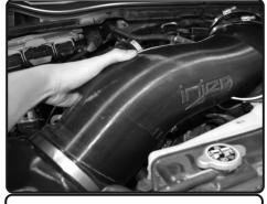
**30.** Install the intake tube and adjust for best fitment.
