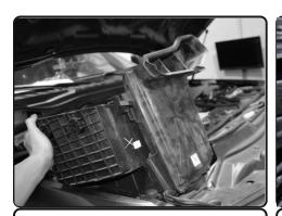
**13.** Remove the OEM battery tray out of vehicle.
