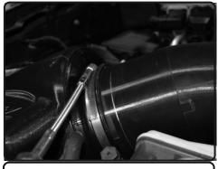
**31.** Once the tube is adjusted, tighten the clamp on the filter and turbo side.
