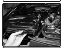
**21.** Install the Air box to the front of vehicle. This is the air box's new position and the battery will sit behind the air box.
