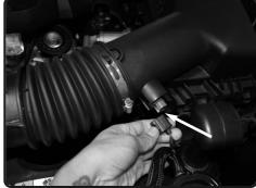
**3.** Disconnect the air intake sensor harness and then twist the air temp sensor to remove it from the air box assembly.
