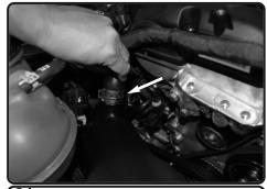
**21.** Re-connect the diverter valve return line to the port on the Injen intake tube use the factory tension clamp to secure it.
