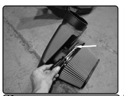
**13.** Place the filter onto the Injen plenum and then secure the clamp
