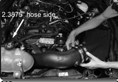
**19.** Place the intake tube into position. Slide the 2.3875" coupler onto the turocharger and then slide the 4.5" hump hose over the plenum. Adjust the intake for best fitment and then secure the clamps
