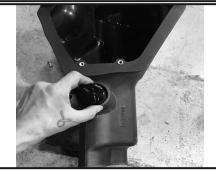
**9.** Install the Filter Minder plug into the Filter Minder pod on the lower air box assembly
