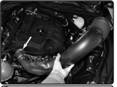
**7.** Loosen the clamp on the factory air duct on the turbocharger end and then remove the entire factory air duct from the engine bay.
