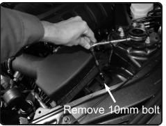
**2.** Remove the 10mm bolt from the side of the stock OE air box.
