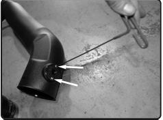
**16.** Place the machined air temp sensor adapter onto the tube and secure it with 2-M4X16 bolt.
