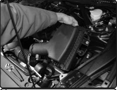
**4.** Loosen the clamp on the factory air duct and then firmly lift the airbox from the engine bay.
