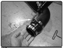
**18.** Place the 2.3875"-3.0" step hose and #48 and #36 clamps onto the smaller end of the Injen intake tube and only secure the clamp on the 3.0" side for now.
