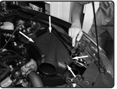
**15.** Place the Injen plenum onto the Injen lower air box assembly and use 4-M6X30 bolts to secure the plenum to the lower air box.
