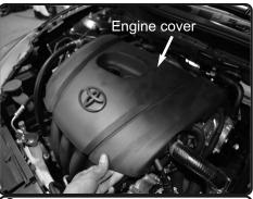
**2.** Lift up and remove engine cover.
