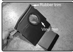
**12.** Install the rubber trim to the top of the heatshield. Install the vinyl trim to the hole in the center of the heatshield.
