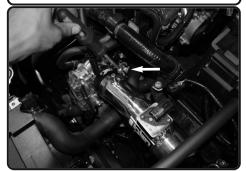
**21.** Adjust and position tube to the center hole of heatshield. Secure and tighten clamps on throttle body.
