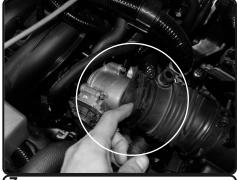
**7.** Pull back the intake tube from the throttle body.
