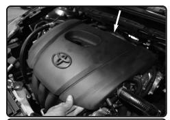
**25.** Re-install engine cover. Re-connect battery..
