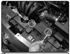
**3.** Loosen the 2 screws holding in the airbox using 10mm socket and ratchet. Save 1 screw for later install.
