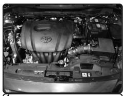
1. Stock intake system shown. <u>Disconnect battery</u>, <u>vehicle may throw Check Engine Light if not disconnected</u>, <u>MAF sensor has constant voltage running even with vehicle off</u>.
