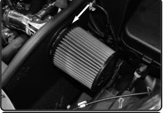
**24.** Install the filter to the intake tube, secure and tighten using 8mm nut driver.
