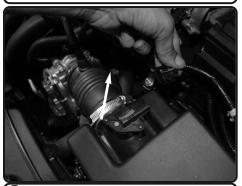
**5.** Disconnect MAF sensor harness and pull away from airbox.
