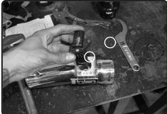
**10.** Secure and install into the new injen intake tube using M4 screws. Tighten using 2.5mm allen key.
