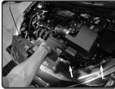
**8.** Lift up and remove the complete stock intake system out of vehicle.
