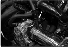
**22.** Install the provided 10mm hose to the fitting on intake tube. Secure the OEM plastic crankcase line to the 10mm hose.
