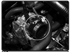
19. Install the straight hose with clamps provided to the throttle body. Tighten clamp on throttle body.
