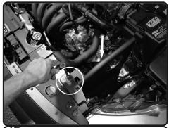
**17.** Secure and tighten the heatshield using 10mm socket or wrench.
