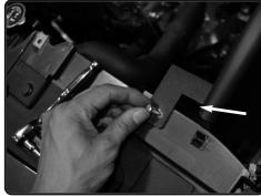
**16.** Now install M6x16mm hex screw to the tab and secure to the OEM airbox insert from step 3.
