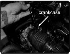
**4.** Lift up and remove the crankcase line from intake tube.
