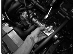
**20.** Install the intake tube into vehicle. Position the tube to the throttle body.
