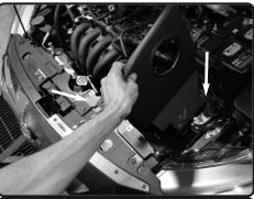
**14.** Position the heatshield into the vehicle, Do not secure.
