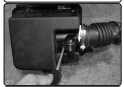
Loosen and remove the MAF sensor out of air box using phillips screwdriver.
