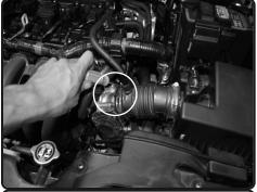
**6.** Loosen the clamp on the throttle body using 7mm socket and ratchet.
