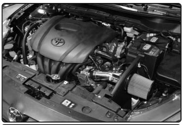
Congratulations! You have just completed the installation of this intake system. Periodically, check the alignment of the intake, normal wear and tear can cause nuts and bolts to come loose.
