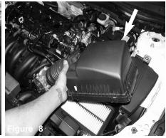
Un-clip the upper half of the air box and remove the assembly.
