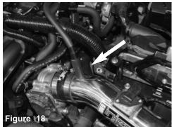
Now install the hose assembly from step 11 and connect Now connect the MAF sensor harness. to the intake tube fitting.
