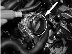
Install the straight hose with clamps to the throttle body. Tighten the clamp on the throttle body only
