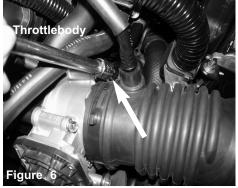
Loosen the clamp on the throttle body using 10mm socket and ratchet. Pull back crankcase line from intake tube.
