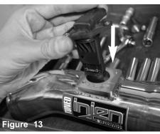
Install the MAF sensor into the intake tube and secure using provided M4 screws.
