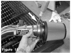
Install the filter to the intake tube. Tighten using 8mm nut driver.
