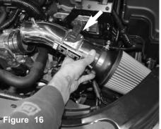
Now install into vehicle and position the intake tube to the hose on throttle body.
