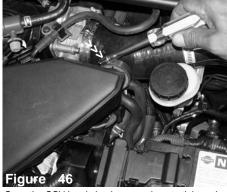
Once the CCV box is in place, continue to tighten the hose clamp over the CCV box outlet.
