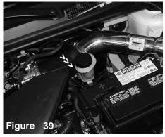
The upper intake tract is firmly pressed into the throttle body hose. Note: Prior to tightening the flange nut, be sure to leave 1/2" space around the reservoir bottle
