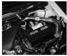
Once the intake bracket is sitting flush on the vibramount stud, continue to semi-tighten the power-band located on the throttle body.
