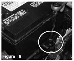
Loosen the m8 bolt located on the tray bracket, once the bolt has been loosened, this will allow the base of the battery to un-wedge itself from the tray.
