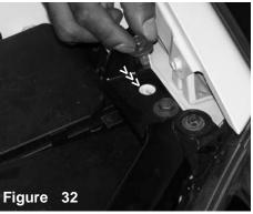
The m8 screw is now removed from the bracket as shown above.
