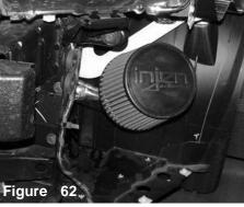
Once the intake has been butted up against the filter stop, continue to tighten the filter neck clamp.
