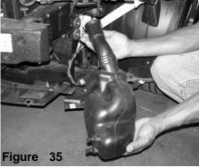
The resonator box is now out of the fender well
