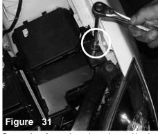
Remove the m8 screw located over the metal bracket that holds the fuse box in place.
