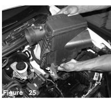
The air box cleaner is now ready to be pulled out from the engine compartment.
