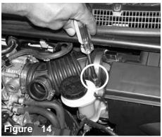
Loosen the hose clamp that connects the air intake duct to the air box cleaner.
