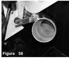
The intake bracket is shown aligned to the vibramount stud.
