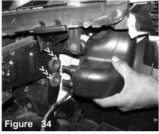
Pull the plastic resonator box from the grommets and pull the resonator box down and out of the bumper and fender well.
