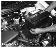
Place the plastic battery tray over the metal battery holder and set the battery back to its original location
