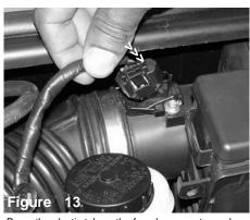
Press the plastic tab on the female connector and pull the electrical harness clip from the mass air flow sensor.
