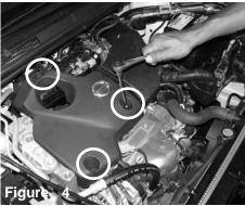
Loosen all three m6 bolts located on the engine cover as shown above.
