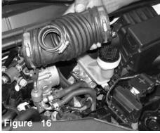
Once all three clamps have been loosened, continue to remove the air intake duct from the throttle body and the air box cleaner.
