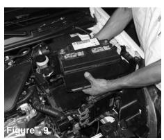
Remove the battery cables and carefully pull the battery out of the engine compartment for now.
