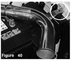
The lower intake bracket is aligned to the vibramount stud as shown above.
