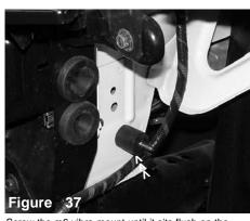
Screw the m6 vibra-mount until it sits flush on the frame.
