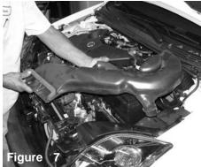
Once you have pulled plastic clips out, continue to pull the factory air scoop out of the engine compart-
