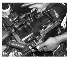
Once you have removed the air box cleaner from the engine compartment, continue to replace the metal battery tray back to its original location.
