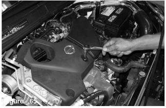
Place the plastic cover over the engine and use the stock bolts to fasten the cover over the intake manifold.
