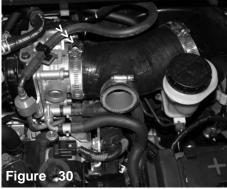
Once the silicone throttle body hose has been pressed over the throttle body, continue to semi-tighten the clamp over the throttle body for now.
