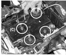
Loosen and remove all four m8 bolts from the battery tray as shown above. Start by removing bolt (A) from the metal battery tray.
