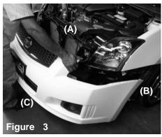
Remove all four clips on top bumper (A), two m6 bolts under the fender well(B), six phillips screws and five clips located under the bumper (C). Now carefully pull the bumper away from the frame.
