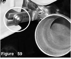
The m6 flange nut and fender washer is used to fasten the intake bracket to the vibra-mount stud.
