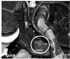
Now that the tray has been lifted out of the way, continue to loosen the m6 bolt located on the corner of the air box.
