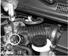
Loosen the hose clamp located on the throttle body.
