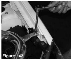
Fasten the m6 flange nut and fender washer on the vibra-mount stud.
