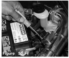
Use the stock bolts to fasten the mass air flow sensor to the sensor adapter.
