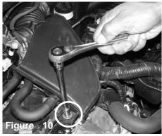
Loosen and remove the m6 bolt located on the CCV box edge.
