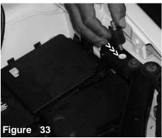
Align and screw the m8 vibra-mount into the fender well bracket as shown above.
