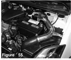
The primary intake and 3" hose is now properly aligned. Again, to avoid any damage to the reservoir bottle, allow a 1/2" gap between the intake and the reservoir bottle.
