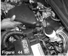
Press the CCV box port into the silicone hose inlet. Position the CCV box in place until it sits level with the engine.
