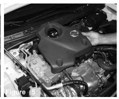
Once all three bolts have been removed, continue to pull the plastic cover out of the engine compartment.
