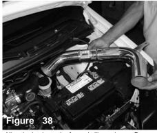
Align the intake to the formed silicone hose. Press the intake into the silicone holes while aligning the intake bracket to the vibra-mount stud.
