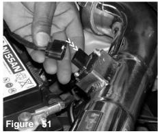
Press the electrical sensor clip over the mass air flow sensor until it snaps in place.
