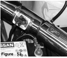
The electrical sensor clip is firmly pressed over the mass air flow sensor.
