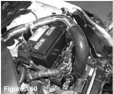
The 3" silicone hose is used to connect the upper and lower air intake tracts. Once all intake tracts have been aligned continue to semi-tighten the
