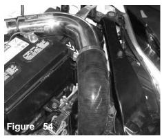
Once you have inserted the front end into the opening, continue to press the top end into the intake end. Semi-tighten the hose clamp for now.
