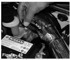
insert the mass air flow sensor into the machined sensor adapter located on the intake.
