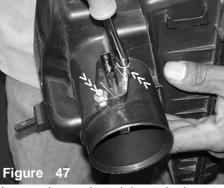
Loosen and remove the two bolts securing the mass air flow sensor to the sensor housing.
