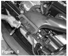
With the use of a screwdriver, insert the head under the clip, pop the plastic clip up and pull the entire clip out.
