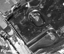
Bolts (C) and (D) are removed next. This will now give you access to the last m6 bolt securing the air box cleaner.
