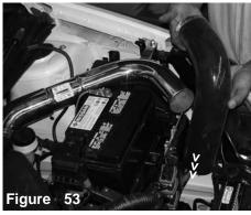
Insert the large 3" silicone hose into the cavity between the battery and the radiator.
