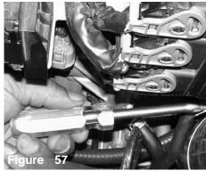
The lower intake tract is inserted into the engine compartment and pressed into the lower 3" silicone hose while aligning the intake bracket to the vibramount.
