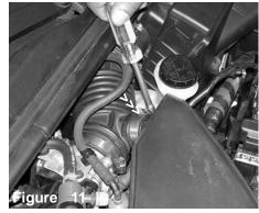
Loosen the hose clamp that fastens the CCV box port to the air intake duct.
