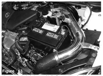
Align the entire intake for best possible fit. Once you have align the intake, continue to tighten all nuts, bolts and clamps.
