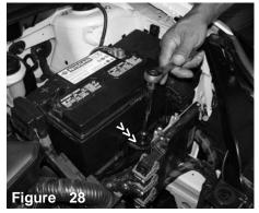
The m8 bolt on the metal battery tray is now fastened.
