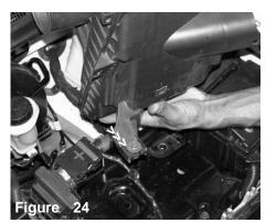
The m6 bolt has been removed, continue to pull the entire air box cleaner from the engine compartment.
