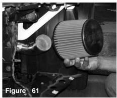
Align and press the filter neck over the intake. intake end will butt up against the filter stop.
