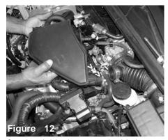
Once the m bolt has been removed and the hose clamp has been loosened, continue to pull the  $\ensuremath{\mathsf{CCV}}$ box away from the air intake duct.
