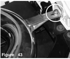
The flange nut and fender washer is sitting flush over the vibra-mount stud.
