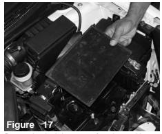
Remove the plastic battery tray from the metal battery holder, this will give you access to the five bolts under the plastic tray.
