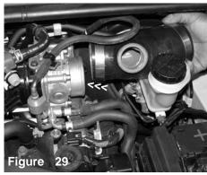
Place the three power-bands over the throttle body silicone hose and align it to the throttle body port.
