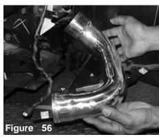
Insert the last intake tract into the bumper area and into the engine compartment.
