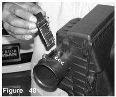
Once both bolts have been removed, continue to pull the mass air flow sensor out of the sensor housing.
