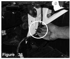
Align the m6 vibra-mount to the pre-tapped hole located on the frame
