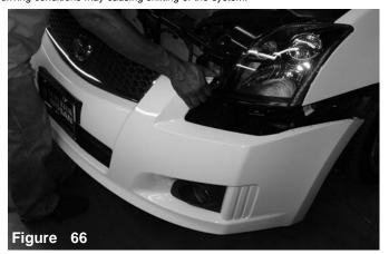
Replace the front bumper back to its original position. Start the engine and allow 5 to10 minutes for the ECU to readjust to the new calibrated and free flowing intake system.
