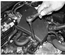
Align the plastic brace to the mounting plate and use the stock bolt to fasten it in place.
