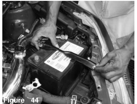
Figure 41 Once you have installed the intake, continue to re-install the battery back to its original location.
