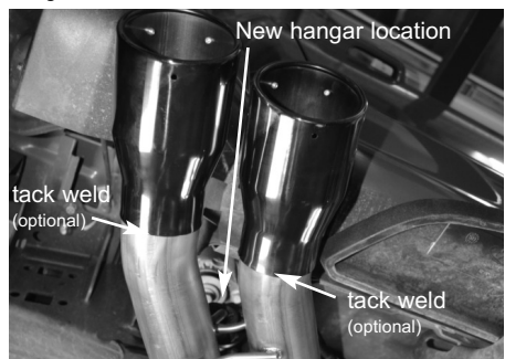
Figure 7 Once exhaust is adjusted to proper fit and clearance, tighten all bolts and screws. Install the provided injen black chrome tips and tighten using allen key. For a more secure fit, you can tack weld bottom of tips so they will not come off.
