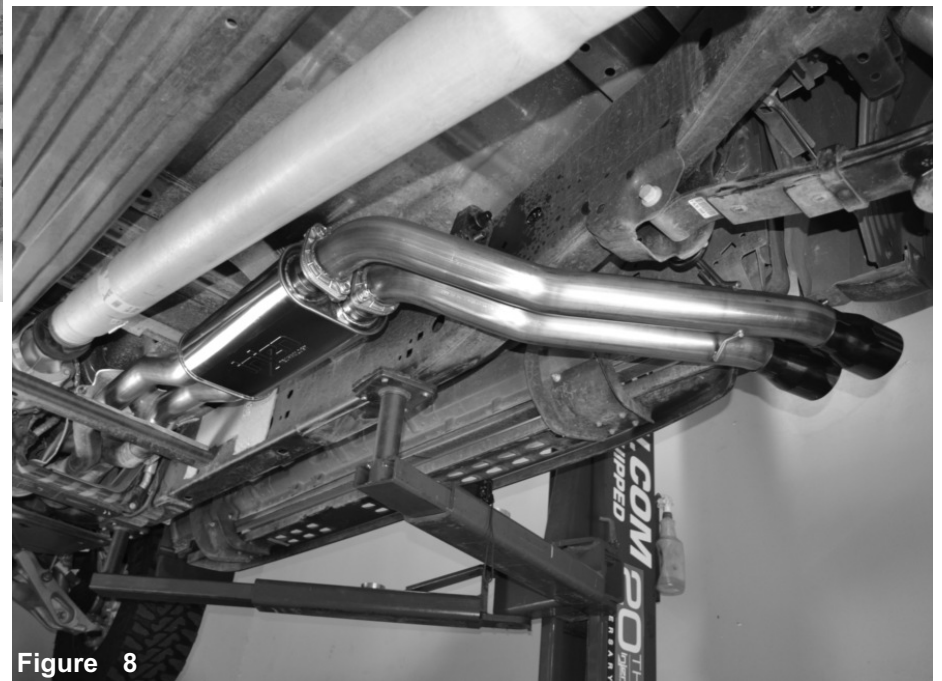
Figure 6 Now install the rear section and secure the flanges using provided M10 bolts and nuts with 3" gaskets. Snug fit and do not tighten. Secure to the rubber hangers.
