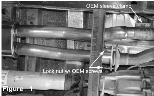
Figure 1 Remove the stock exhaust from vehicle. Install the front section. USE the OEM sleeve clamp on the one side of exhaust. Other side of exhaust, use OEM screws and provided lock nuts and secure. Snug fit exhaust. Do not tighten.
