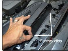
**28.** Re-install the factory retaining rivets from step 2. to the injen scoop and secure. Re-install bumper cover and Re-connect Battery.
