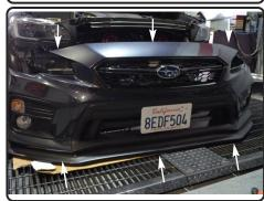
**7.** Loosen and remove the front bumper cover for the installation of the injen intake system.
