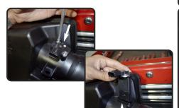
**9.** Loosen the 2 screws holding in the MAF sensor. Now lift up the MAF sensor and remove.
