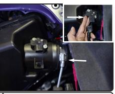
**4.** Disconnect the MAF sensor harness. Loosen
