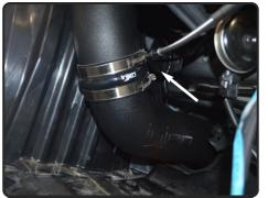
**25.** Now secure and tighten all clamps on the intake system using 8mm nut driver.
