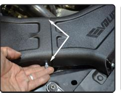
**27.** Secure the scoop to the airbox using provided M6 socket cap screws. Tighten using allen key.
