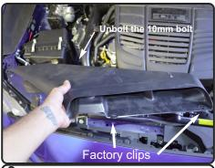
**2.** Remove the two plastic retaining rivets from the air scoop and remove scoop from engine bay. Save for later install. Loosen the 10mm bolt holding in the lower part of the air box to the vehicle frame.
