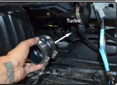
**10.** Install the provided 3" hump hose with clamps provided to the turbo. Tighten the clamp on turbo side only.
