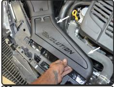
**26.** Install the scoop to the intake system and attach to the inside of the air box.
