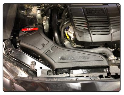
Congratulations! You have just completed the installation of this intake system. Periodically, check the alignment of the intake, normal wear and tear can cause nuts and bolts to come loose. <u>Note: Check clearance and adjust</u> <u>if needed! Failure to check the alignment and adjust the intake can</u> <u>cause damage that will void the warranty. Injen Technology is not re-</u>
