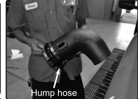
**13.** Place the 5.00" hump hose and two #80 clamps onto the big end of the Injen intake tube
