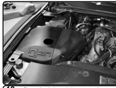
**12.** Drop the Injen air box onto the grommets from figure 11. Make sure the two mounting nipples underneath the Injen air box goes directly into the grommets.
