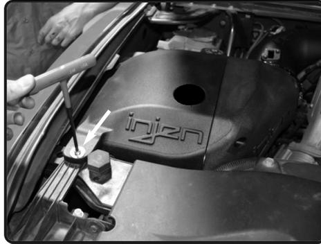
**15.** Place a M6X20mm button head bolt into the Injen air box mounting bracket. Secure the bolt to the chassis.
