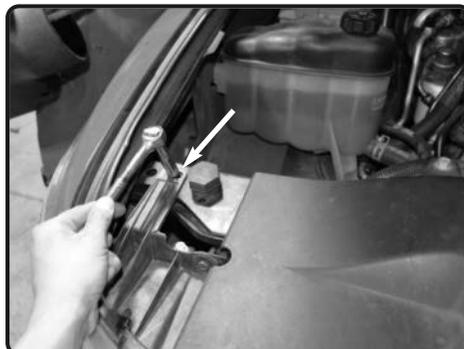
**10.** Use a 10mm socket/ratchet to remove the 10mm bolt from the passenger-side headlight.
