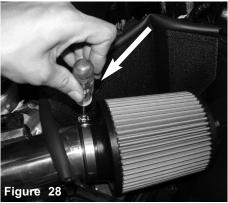
Install the filter to the intake tube. Tighten using 8mm nut driver.
