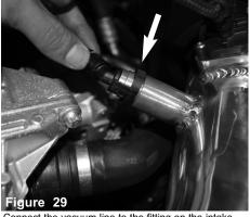
Connect the vacuum line to the fitting on the intake tube. If there is no crankcase line, attach the vinyl cap to the fitting and cap off.
