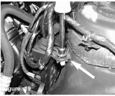
Loosen the screw on the bracket using 8mm nut driver. Save screw for later use.
