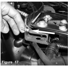
Install the hex screw with fender washer to the support brace T-cutout.
