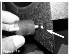
Attach the vibra mount to the thredded fitting on heat shield.
