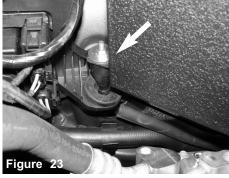
Now secure the stand off stud to seat in the factory grommet of the stock air box location.
