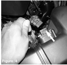
Disconnect the MAF sensor harness. Disconnect the vacuum line from air box. Disconnect vacuum line.
