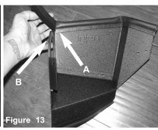
A) Attach the 19"L rubber trim to the top of the heat shield You can cut a notch into the corner for easier install. Attach 8.5"L rubber trim to bottom of shield.
