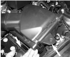
Lift up air box from the factory grommets holding in place.
