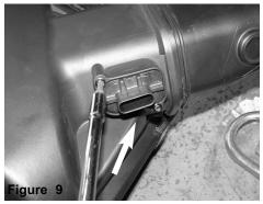
With T20 torx bit loosen the screws holding in the MAF sensor.  $\,$
