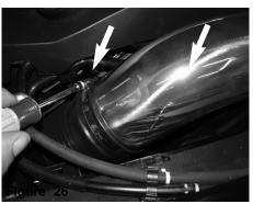
Tighten the clamp on intake tube side, reposition and tighten if tube comes close to the radiator shroud.
