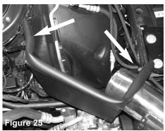
Position for best fit. Tighten the 2 points and secure. Verify the stand off stud is correctly seated.
