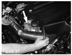
Install the intake assembly into the vehicle and position.
