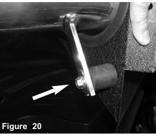
Install the tube into heat shield. Secure the bracket using nut and fender washer to the vibra mount, Do not Tighten.
