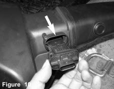
Remove the MAF sensor from the intake tube.
