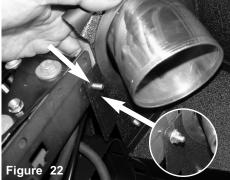
Hold the back of screw from step 18 and secure to heat shield. Secure using provided M6 nut. Do not tighten
