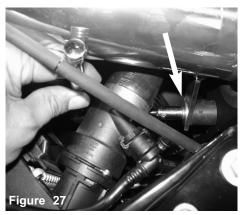
Tighten and secure the bracket on intake tube using 10mm socket and extension.
