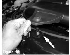
Lift up the intake tube and pull grommet away from the fitting on radiator support.
