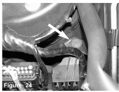
Secure the remaining tab using screw from step 19. Secure and tighten.
