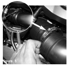
Loosen the clamp on the intake tube and pull back the tube from the factory sleave.
