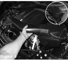
Lift and remove the complete air box out of vehicle. IF EQUIPPED: Remove the supply module cover for heatshield to fit. This cover will no longer be used
