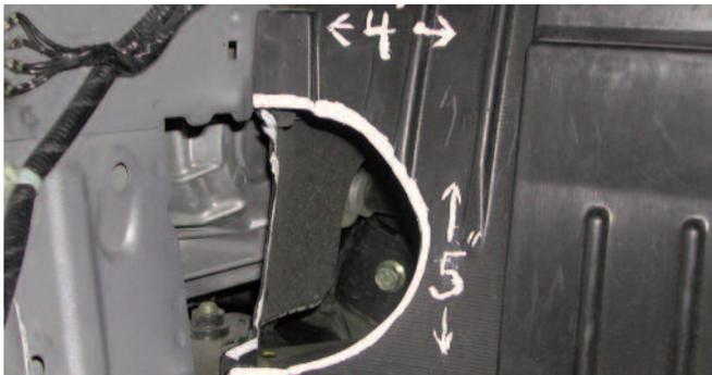
Once the tank has been removed cut a 4" x 5" open on both sides of the splash guard. This will allow access to the bumper area for the filter.
