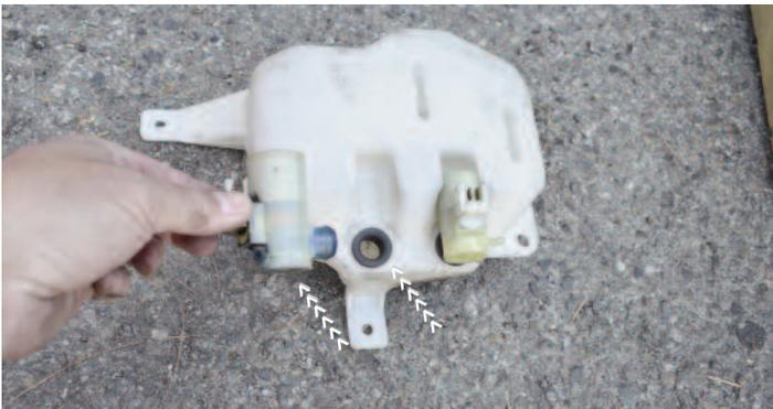
Remove the two OEM grommets and pumps from the OEM reservoir
