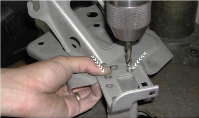
Remove the battery tray from the engine bay. Flip the battery tray upside down and drill out the two spot welds securing the harness bracket to the battery tray.
