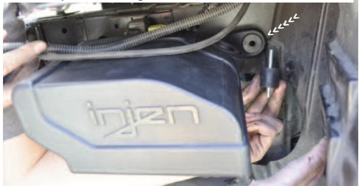
Use the long stud end of the vibra mount to secure the Injen reservoir bottle to the chassis. Continue to secure the other two remaining bolts
