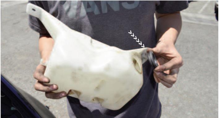
Remove the OEM grommet from the OEM reservoir bottle
