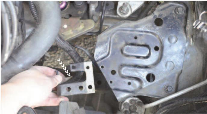
Once the spot welds are drilled out, remove the bracket from the battery tray and reinstall the battery tray to its original location.
