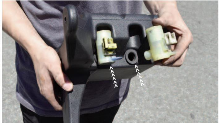
Install the OEM pumps and grommets onto the Injen reservoir
