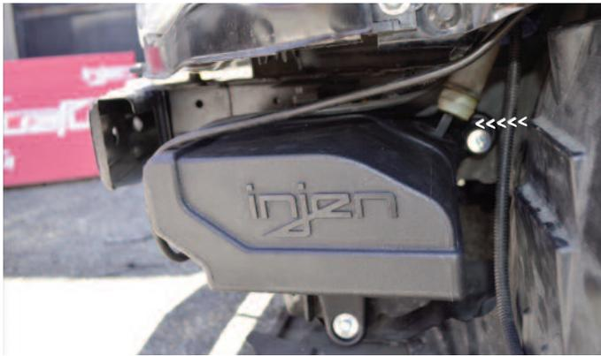
Push the OEM pour spout tube into the large grommet
