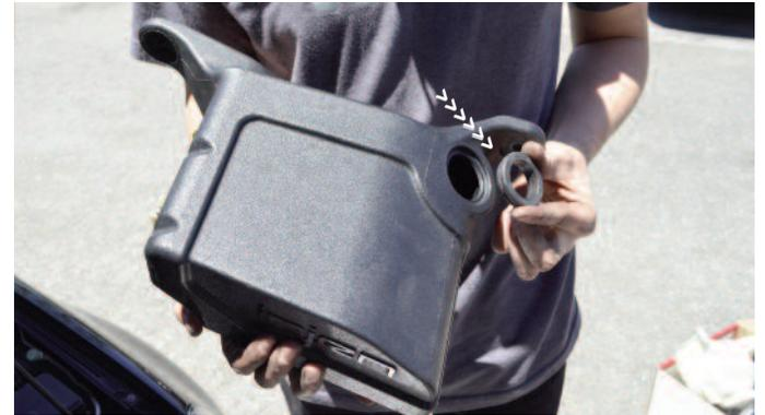
Install the OEM grommet onto the Injen reservoir bottle
