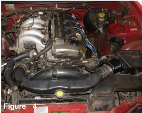
Figure 5 Loosen the clamp on the throttle body intake duct.
