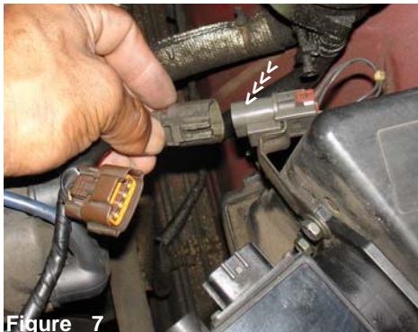
Figure 7 Depress the tab on the harness clip connected to the air temperature sensor and remove the harness clip.
