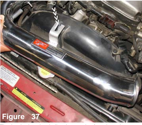
Figure 38 The air intake is in place and ready to be secured.
