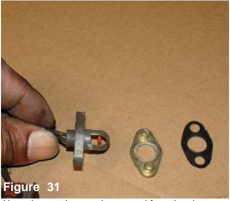
Figure 28 Loosen the two small screws from the air temperature sensor that fastens it to the upper air box cleaner.
