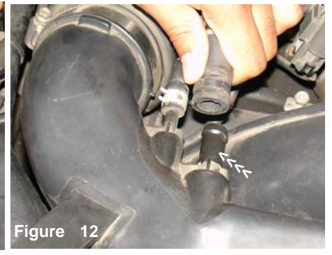
Figure 9 Once you have removed the tension clamp, continue to disconnect the CVC breather hose from the air intake port.
