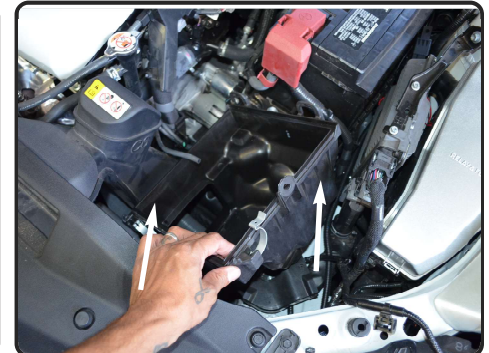
8. Lift up and remove the lower part of air box out of vehicle. Leave the front OEM ram scoop in vehicle.
