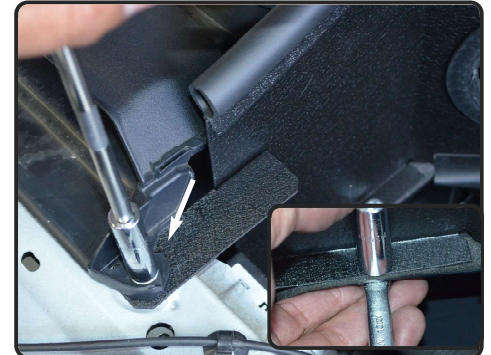
20. Now secure and tighten all the screws and nuts using socket or wrench.
