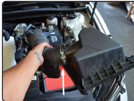
7. Un-clip the upper half of the air box and remove the stock intake assembly out of the vehicle.
