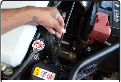
21. With provided 1/8" plastic fitting coupler and 3mm hose from step 5. Connect the OEM vacuum line.
