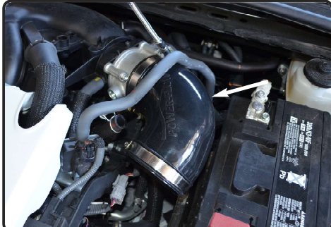
22. Install the 3-1/2" elbow hose with clamps provided to the throttle body.
