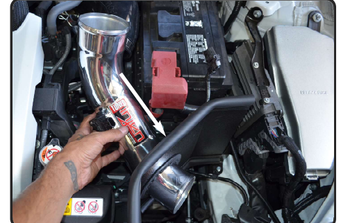
24. Install the intake tube through the hole on heatshield and position to the coupler on throttle body.
