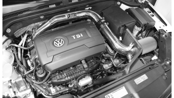
Figure 31 Now tighten the clamp on the turbo side using 8mm nut driver.
