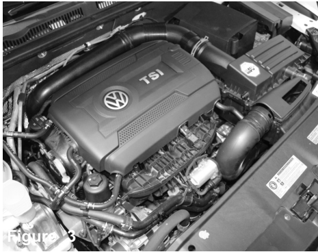
Figure 3 Stock box shown in this picture, if desired remove the engine cover for easier installation.
