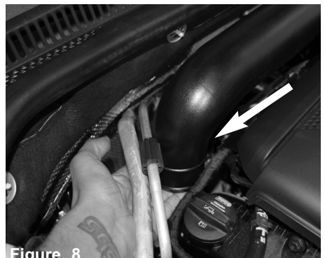
Figure 8 With pliers, carefully pull the intake tube out
