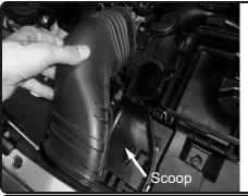
**3.** Carefully un-clip the the push clips and remove the scoop from vehicle.
