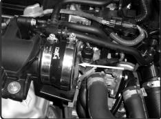
**14.** Attach the hose with clamps to the intake tube.
