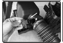
**8.** Loosen the 2 screws holding in the MAF sensor and remove. Save screws for later install.
