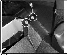
**18.** Secure the heatshield to the original air box bracket mounting points using OEM screws from step 6.
