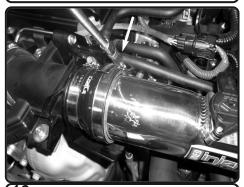
**16.** Rotate and position. Tighten all clamps using 8mm nut driver.
