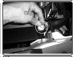
**19.** Secure the side of heatshield using provided M6 fender washer and screw. Secure and tighten.
