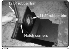
**10.** Add the 12.5 Rubber trim to the top of the heatshield, and the 11.5 rubber trim to hole on heatshield. *Notch corners for easier installation with pliers.*
