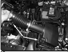
**5.** Now un-clip the upper part of the air box assembly. Lift up and remove from the vehicle.
