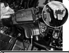
**6.** Carefully lift up corner of air box, this will require some force. Remove the bottom half of the air box out of vehicle. Loosen the 2 bolts holding in the air box bracket and remove bracket. Save bolts for later install.
