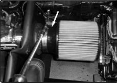
**21.** Install the air filter and tighten using 8mm nut driver.
