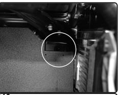
**13.** Make sure the heatshield bracket with grommet is seated on the stud.
