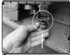
**7.** Now remove the OEM grommet from the air box. This will be used on new injen heatshield.
