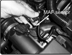
7. Disconnect the MAF sensor harness and pull harness cable from the air box.
