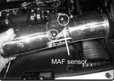
**9.** Now install the MAF sensor into the new injen intake tube. Secure using the OEM screws from the previous step.
