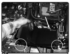
**12.** Install the heatshield and position the brackets to the oem air box mounting locations.
