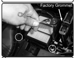
**4.** Loosen the 2 bolts holding in the lower part of the air box.
