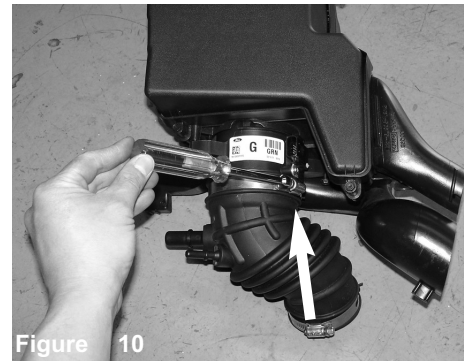
Figure 10 Loosen the clamp on the air box using 8mm nut driver and remove the stock intake tube.
