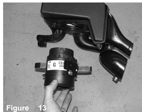
Figure 13 Carefully remove MAF sensor housing from air box.
