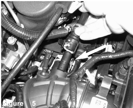
Figure 5 Disconnect the crank case line from the stock intake.
