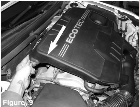
Figure 9 Lift up engine cover and remove from vehicle.
