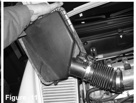
Figure 11 Un-clip upper half of air box and remove.
