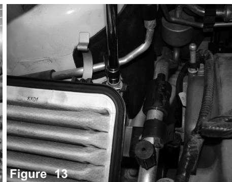
Figure 13 With 10mm socket and ratchet, loosen and remove the bolt holding in A/C line and air box.
