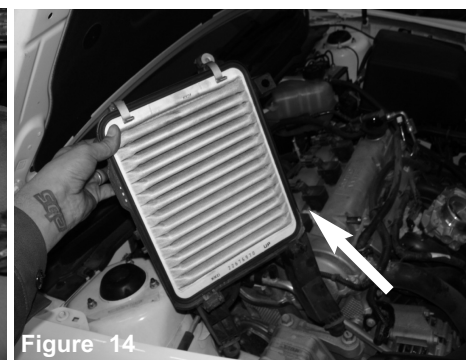
Figure 14 Carefully maneuver the bottom half of air box out of vehicle. Note: becarefull and not damage the A/C line. Re-install the bolt from previous step and secure the A/C line.
