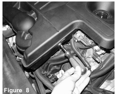
Figure 8 With long 8mm nut driver, loosen the clamp under the engine cover on throttle body.
