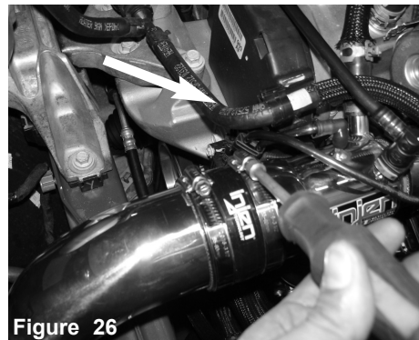
Figure 23 For cold air application, remove the air filter and install the provided 3" hose with clamps to the upper intake assembly. Tighten on the tube only.
