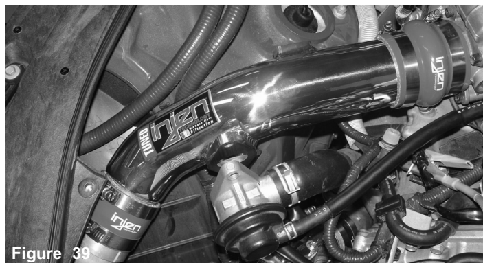
Figure 39 Position for the best possible fit and tighten all the clamps on the intercooler pipes.
