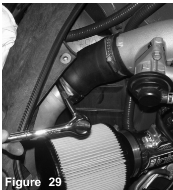
Figure 29 Figure 30 Installation of the upper intercooler pipes, Note: installation is the same for both sides, photos are of passenger side only. Loosen the clamps on both sides of intercooler pipes using 8mm nut driver or socket with ratchet.
