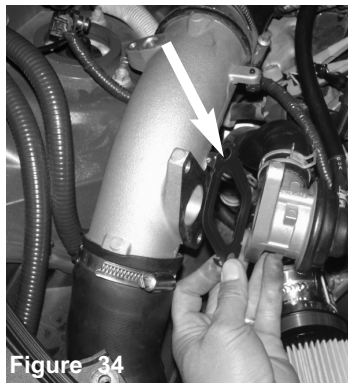
Figure 33 Figure 34 Loosen the 2 bolts holding in the blow off valve using 12mm socket or wrench, pull back and save the factory gasket.
