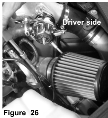
Figure 25 Figure 26 Install filters and secure using 8mm nut driver. Tighten all remaining clamps.
