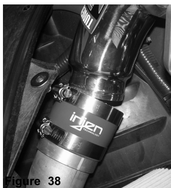
Figure 37 Figure 38 Attach the 2-3/4" hump hose to the new intercooler pipe, install the intercooler pipe and slide the hump hose on to the throttle body with clamps provided.
