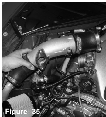
Figure 35 Figure 36 Now carefully pull back the sensor harness line, and remove the factory upper intercooler pipe. Install the 2-3/8" hose to the factory intercooler pipe.
