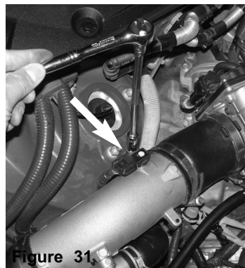
Figure 31 Figure 32 Loosen the screw holding in the temperature sensor, save screw for later install. Pull out the temperature sensor.
