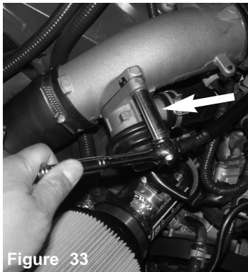
Figure 33 Figure 34 Loosen the 2 bolts holding in the blow off valve using 12mm socket or wrench, pull back and save the factory gasket.
