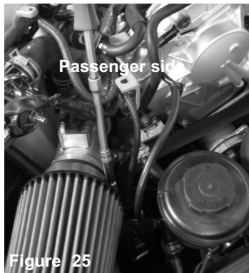
Figure 25 Figure 26 Install filters and secure using 8mm nut driver. Tighten all remaining clamps.
