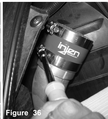
Figure 35 Figure 36 Now carefully pull back the sensor harness line, and remove the factory upper intercooler pipe. Install the 2-3/8" hose to the factory intercooler pipe.
