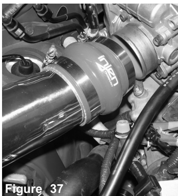
Figure 37 Figure 38 Attach the 2-3/4" hump hose to the new intercooler pipe, install the intercooler pipe and slide the hump hose on to the throttle body with clamps provided.
