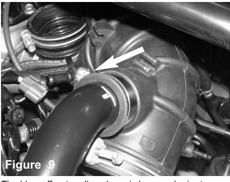
Figure 9 The blow off return line clamp is loosened prior to removing the air box. The hard line is removed from the intake tube.
