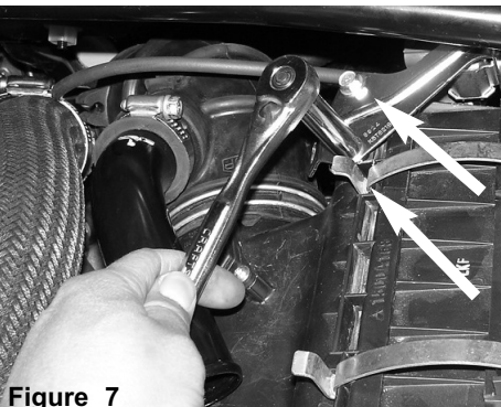
Figure 7 The two bolts on the boost solenoid bracket are loosened and removed from the air box.
