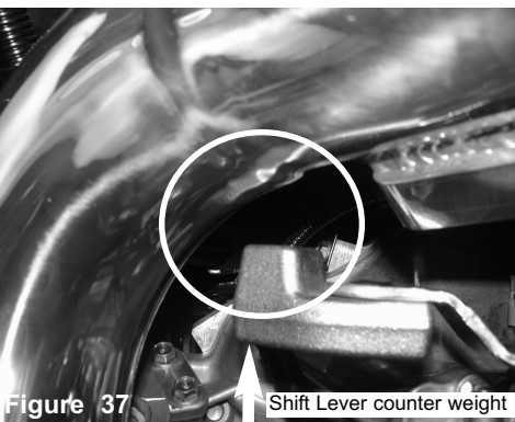
Figure 37 IMPORTANT!!! Place the car in 5th gear and make sure the shift lever counterweight does not come in contact with the intake pipe. Shift lever counter weight should clear pipe as shown in photo
