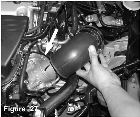
Figure 27 Place two clamps and the 60 degree 2 7/8X3.00 elbow with the 2 7/8" end onto the throttle body
