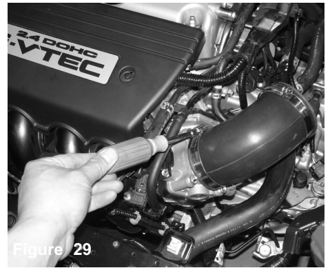
Figure 29 Now tighten only the clamp on the throttlebody side.
