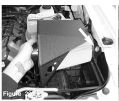
Instal the heat shield assembly into the vehicle and position tab side first.
