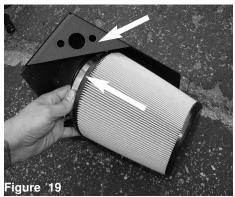
Install the filter to the adaptor and tighten using 8mm nut driver.
