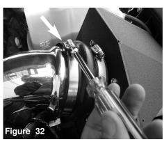
Tighten the clamps on the hump hose using 8mm nut driver.
