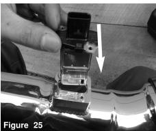
Install the MAF sensor into the new injen intake tube.
