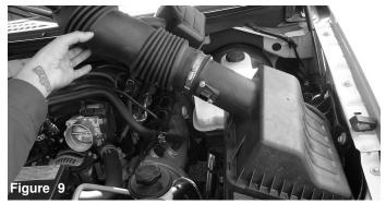
Now, lift and remove the whole intake assembly out of vehicle.
