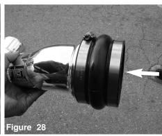
Install the hump hose with clamps to the tube, Do not tighten.
