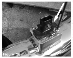
Secure the MAF sensor using provided M4 button head screws and tighten using 2.5mm allen key.
