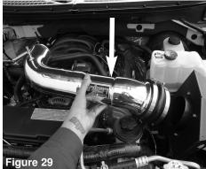
Install the intake tube into the vehicle and position to Slide the hump hose on to the adaptor and position. the throttle body and adaptor.
