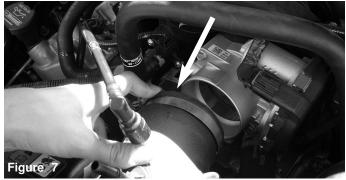
Pull back the intake tube from the throttle body.
