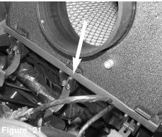
Make sure the heat shield assembly with trim seats in the groove. Position heat shield forward for the tab to align with hole from step 11. Align the tabs to clips.
