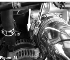
Now tighten the clamps on throttle body using 8mm nut driver.
