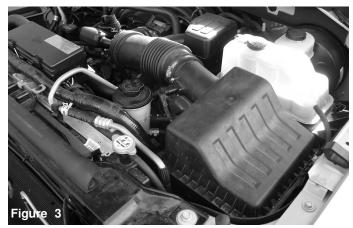
Complete stock intake shown. Disconnect battery before install.
