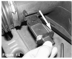
Carefully pull the MAF sensor out and set aside.
