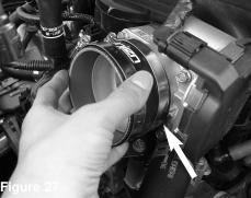
With clamps provided, attach to the straight hose and install to the throttle body.
