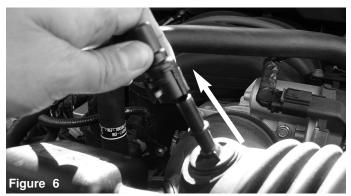
Disconnect the crank case line from stock fitting on intake tube.
