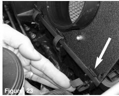
Secure the heat shield and clip to tabs.
