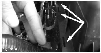
Un-clip the 3 clips holding in upper half of air box and slide back.
