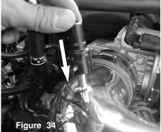
Re-connect the crank case line to the fitting on the new injen intake tube.
