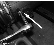
With t20 torx bit, loosen and remove the 2 screws holding in the MAF sensor.
