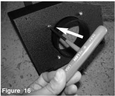
Secure the adaptor using the provided M6 button head screws and tighten using allen key.
