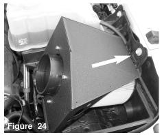
Tighten the bolt using 13mm socket and ratchet. Make sure the heat shield assembly is tight and secure.
