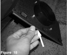
Attach the other vinyl trim to the side with tabs. *Note:* make sure you attach the trim to heat shield to prevent rubbing and vibration.
