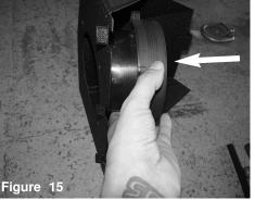
Install the 4" velocity adaptor tot he inside of the heat shield.
