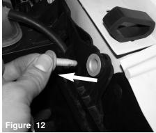
Remove bolt and save for later install.
