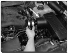
**12.** Place the 4.00" hump hose and 2-#64 clamps onto the Injen intake plenum. Make sure you push the hump hose all the way over to allow room for the intake tube.
