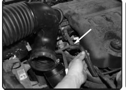
**5.** If your vehicle is equipped with with a vacuum line, disconnect it and place to the side for now.
