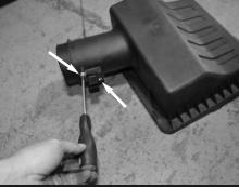
**3.** Remove the two torq screws and remove the MAF sensor from the upper air box assembly
