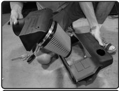
**7.** Once the Filter Minder plug is installed in the upper air box, install the filter onto the Injen air box plenum.
