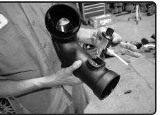
**10.** Place the MAF sensor into the Injen intake tube and secure it with the two M4 supplied screws.
