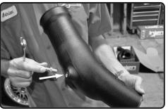
**11.** If your vehicle is equipped with a vacuum line, place the 1/4 NPT 3/8 barbed fitting into the insert on the intake tube. Place the 1/4 NPT plug if no vacuum line is present
