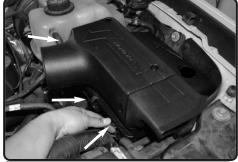
**9.** Install the Injen upper airbox and plenum onto the lower OEM airbox assembly and attach the 3 factory metal clips to secure the Injen air box to the OEM air box
