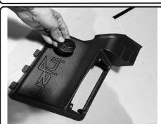
**6.** Place the Filter Minder plug into the hole on the upper air box assembly
