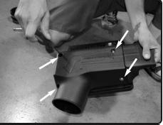
**8.** Use 4-M6X30 screws to secure the plenum to the Injen upper air box.
