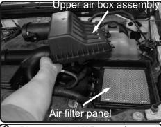
**2.** Disconnect the MAF sensor harness and unclip the 3 metal tabs holding the upper air box to the lower air box. Remove the upper box assembly and air filter panel.
