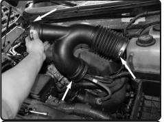
**4.** Loosen the three clamps on the factory Y-air duct and remove it from the engine bay.
