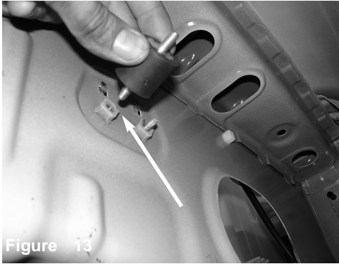
Figure 13 From inside of fenderwell, install male/male vibra mount to threaded fitting and tighten.
