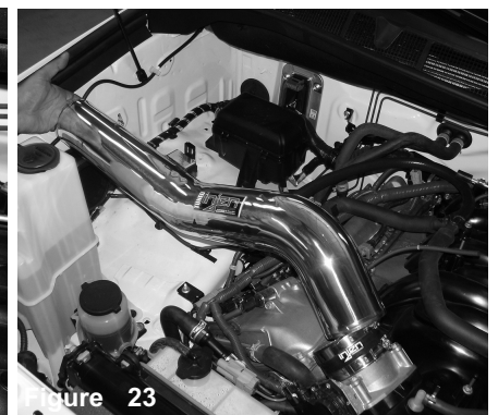
Figure 23 Install intake into vehicle and position.
