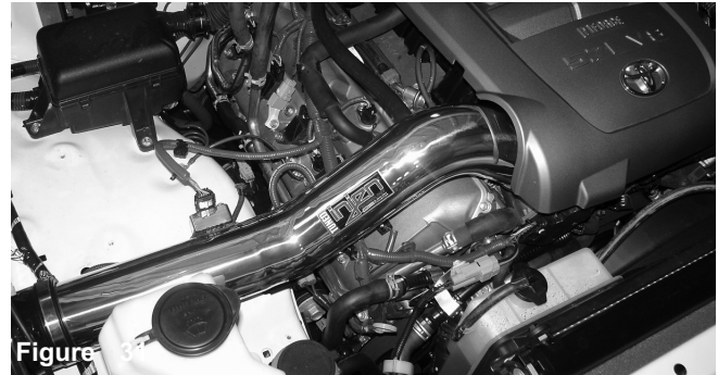
Figure 28 A) Loosen engine cover fitting using 10mm wrench. B) Install male/female vibra mount and secure. C) Re-install fitting to vibra mount and secure.
