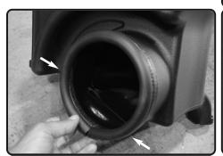
**9.** Install the provided Rubber trim to the hole cut out.
