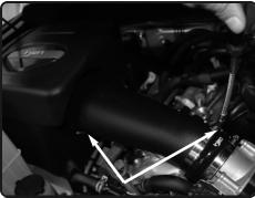
**15.** Adjust the intake for best fitment and then secure all the clamps. Tighten using 8mm nut driver.
