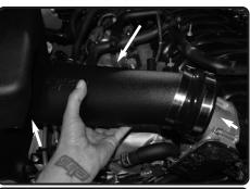
**14.** Insert the Injen intake tube assembly to the vehicle.
