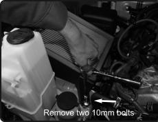
**6.** Locate the 2 bolts holding in the bottom half of the air box, loosen and remove.
