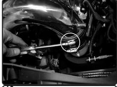
**18.** Secure the hose and tighten clamps using 8mm nut driver.
