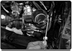
**12.** Tighten the clamp on turbo only.
