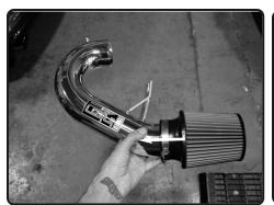
13. Install the filter to the tube.
