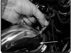
**19.** Connect the vacuum line to the fitting on the intake tube.
