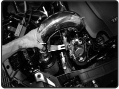
**15.** Install the intake assembly into the vehicle.
