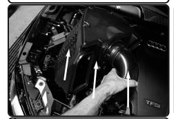
**9.** Carefully lift up and remove the en-tire air box assembly out of vehicle.
