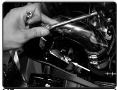
**17.** Tighten bracket using 10mm socket or wrench.
