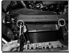
**4.** Locate the 2 bolts holding the front air scoop and remove using T25 torx bit.
