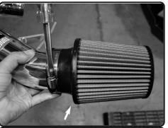
14. Secure and tighten using 8mm nut
