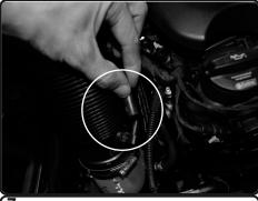
**7.** Pull back the vacuum line from the OEM intake tube.
