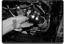
11. Install the provided step hose with clamps provided to turbo.
