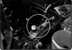
**10.** Now install the provided female/male M6 vibramount to the thredded stud on ve-hicle frame. Secure and tighten.
