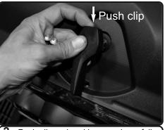
**2.** Push clip on hood lever and carefully remove the lever out of vehicle.
