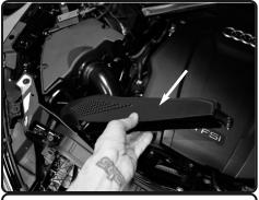
**6.** Remove the ram scoop from vehicle.
