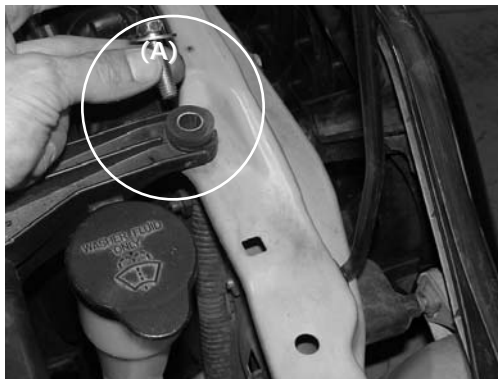
Remove the 10mm bolt located on the cross member. This will allow you to remove the entire air intake box.
