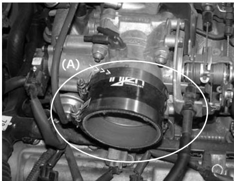
Press the 2 3/4" straight hose over the throttle body, place two .312 bands on the hose and tighten the band on the throttle body side (A).
