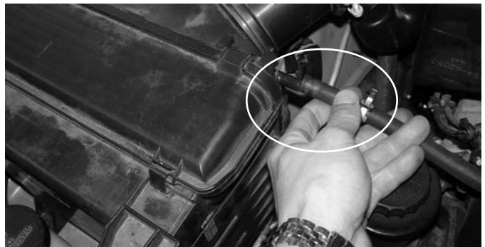
Disconnect the stock 3/8" breather hose connected to the air intake box port. This line will be reused and connected to the first 3/8" port nearest to the filter on the Injen intake pipe.
