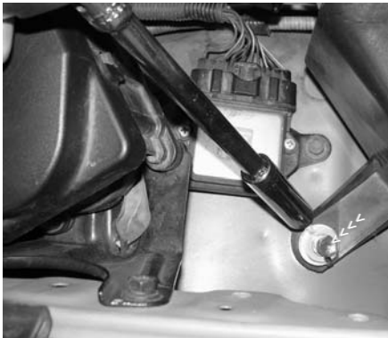
Remove the 10mm bolt by the cruise control box in order to remove the air intake box.
