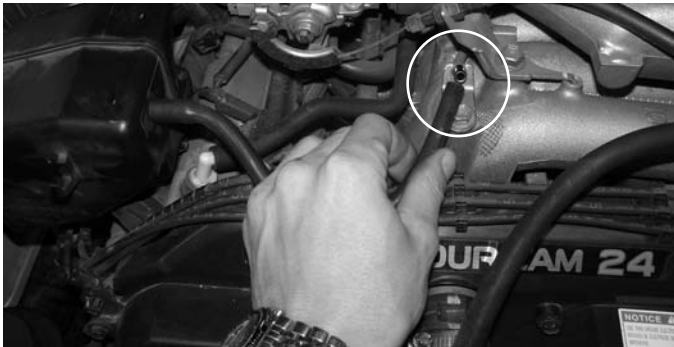
Disconnect the stock 3/8" vacuum line connected to the small intake manifold port. This line will be replaced with the Injen 27" 10mm vacuum hose.
