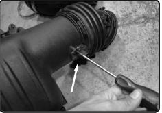
**11.** Loosen and remove the MAF sensor out of the airbox.
