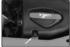
**10.** Install the air box assembly into the vehicle. Secure using OEM screw. Make sure the nipple fitting on back side of injen airbox is seated in the OEM grommet on fender well.
