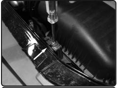
**5.** Loosen the screw holding in the airbox using 8mm nut driver. Save for later install.
