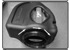
**9.** Once seated, rotate in either direction 1/4 turn till filter locks.
