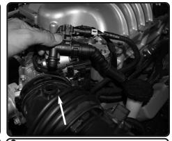
**3.** Pull back crank case line from intake tube fitting.
