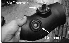
**12.** Install the provided crankcase grommet to the hole cutout on the tube.
