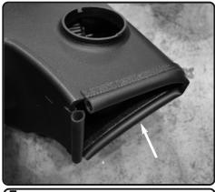
7. Install the provided bulb trims to the bottom of the airbox.
