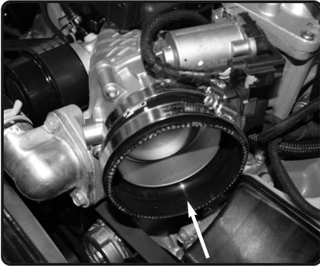
**13.** Install the step hump hose to the throttle body. Install the intake tube and position for fit.
