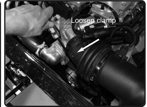
4. Loosen the clamp on throttle body using 8mm nut driver.
