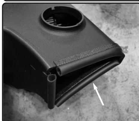
7. Install the provided bulb trims to the bottom of the airbox.
