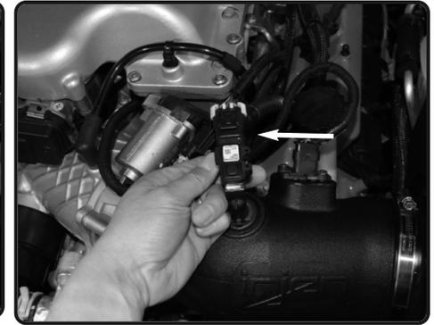
**16.** Secure and make sure the unit is pushed closes to the throttle body. This will clear the hood and not hit.
