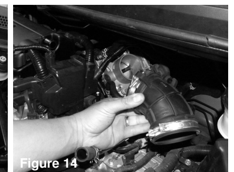
Figure 11 Use a 5.5mm socket and ratchet and loosen the clamp on the lower air box assembly air duct to throttle body. Then continue to loosen the clamp on the throttle body side.
