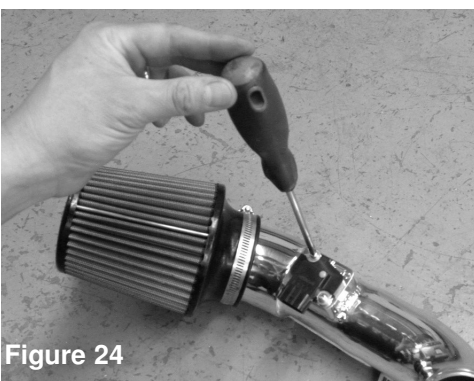
Figure 24 Use a phillips screw driver and tighten the two screws to secure the MAF sensor to the machined MAF sensor pad.
