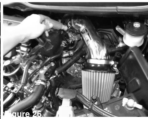
Figure 26 Due to the short length of the intake pipe, it does not require a mounting bracket. Position the intake for best fitment and then tighten the clamp to secure pipe to the throttle body.
