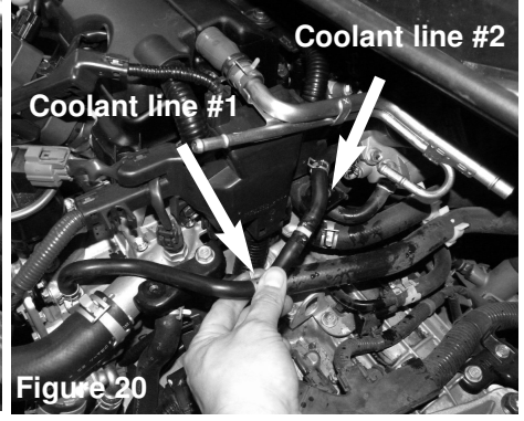
Figure 20 Now connect coolant line #1 to #2
