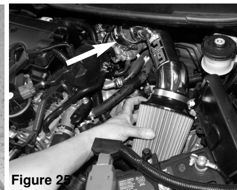
Figure 25 Position the intake pipe into the engine bay and place the end of the intake pipe into the throttle body
