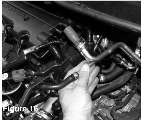
Figure 16 Detach the metal CCV line from the valve cover.
