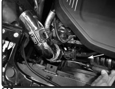
**18.** Install the intake tube ans position for the best fit. Tighten clamp using 8mm nut driver.
