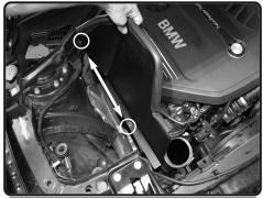
**14.** Install the heatshield into the vehicle and position the 2 grommets to the studs from step 6.
