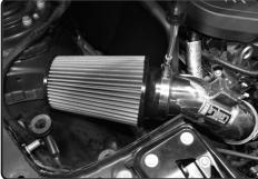
**21.** Secure and tighten the filter using 8mm nut driver.
