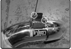
**9.** Install the MAF sensor in the correct direction. Secure using the provided M4 screws. Tighten using 2.5mm allen key.
