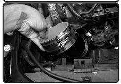
**10.** Install the provided 3.75" with clamps to the turbo.
