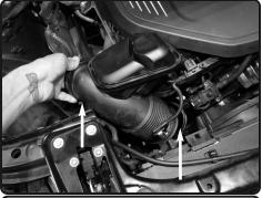
**3.** Loosen the clamp on air box and pull back the intake tube.
