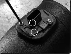
**5.** Install the MAF sensor in the correct direction. Secure using the provided M4 screws. Tighten using 2.5mm allen key.
