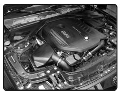
**1.** Stock intake system shown. Lift up and remove engine and the front radiator cover.
