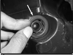
**6.** Remove the factory grommet fitting plug from the bottom of the airbox.
