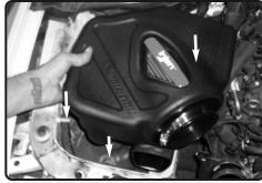
11. Install the injen airbox into the vehicle. make sure the airbox is seated in the OEM locations.
