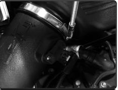
**13.** Position for best fit. Tighten clamp on filter using 8mm nut driver.
