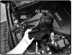
7. Now lift up and pull the entire air box assembly out of the vehicle.
