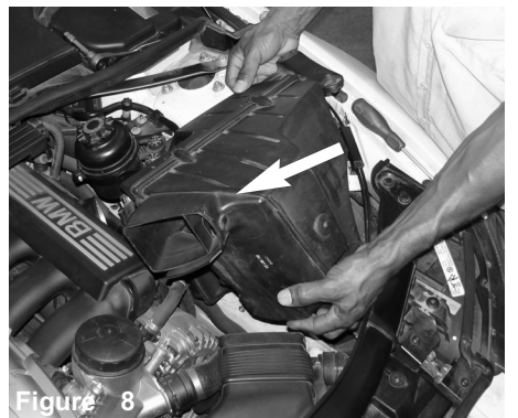
Figure 8 Once both screws have been removed, continue to pull the air box cleaner from the engine compartment.
