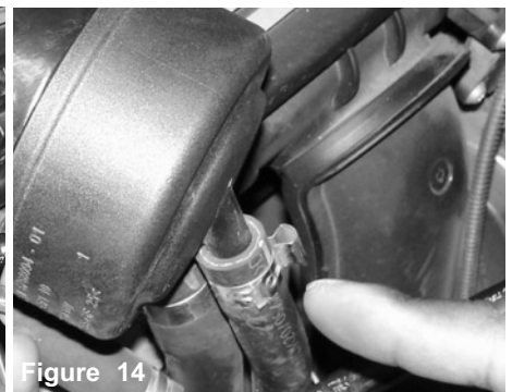
Figure 14 The clamp is now in the correct position, facing to the side. This will prevent any damage to the intake.
