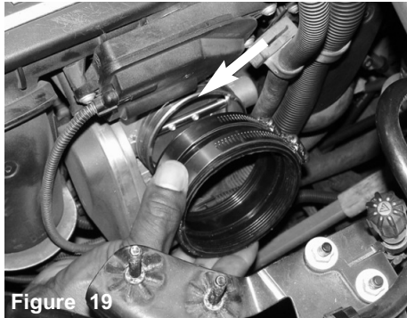
Figure 16 On the 2008-09 128i and 2007-09 328i the vacuum hose is removed prior to loosening the clamp over the throttle body.
