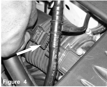
Figure 4 The electrical sensor harness is disconnected.
