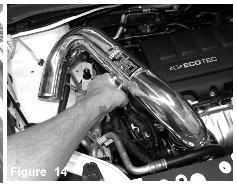
Figure 14 Install the intake tube and position the bracket to the stand off stud, and to the hose.
