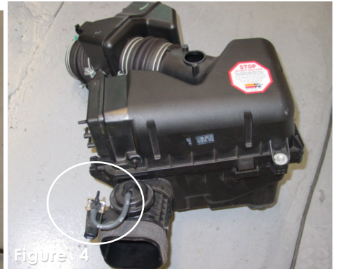
Figure 4 Note, the vacuum switching valve is intact with the air intake box which is no longer used.
