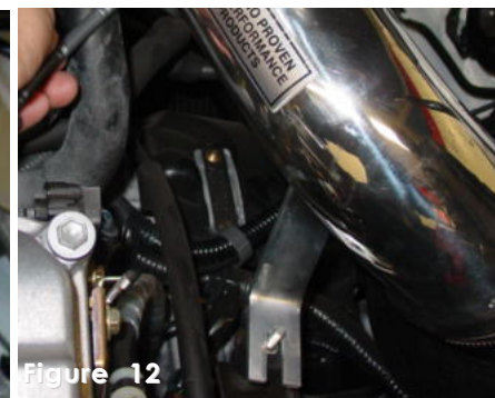
Figure 12 Before the clamp is tightened make sure the bracket on the intake is lined up to the vibra-mount stud. Use the m6 flange nut and fender washer to secure the intake in place.
