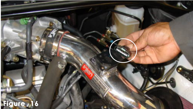
Figure 16 Use the stock self-tapping screws and secure the mass air flow sensor to the machined adapter.
