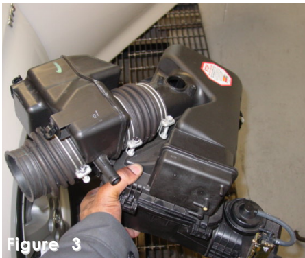
Figure 3 Remove the entire stock air intake box from the engine compartment.
