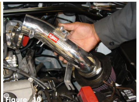
Figure 10 Take the assembled filter and intake and press the top end into the hose on the throttle body.
