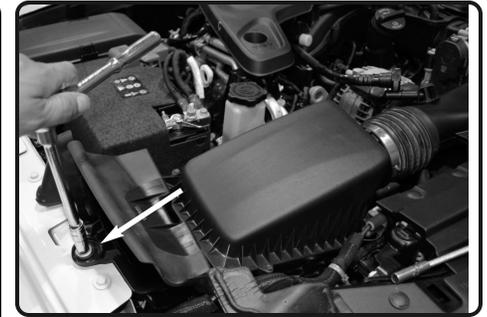
4. On the air box, loosen the bolt holding in the airbox. Loosen bolt and save for later install along with the grommet and crush washer.
