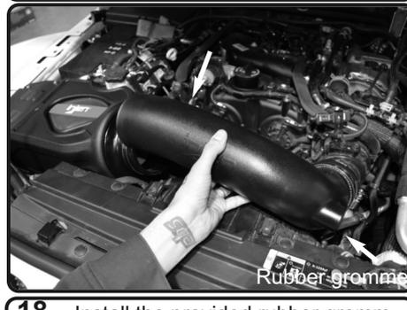
**18.** Install the provided rubber grommet to the intake tube hole. Insert the Injen intake tube into the vehicle. Position tube to the filter and turbo inlet. Position for best fit.
