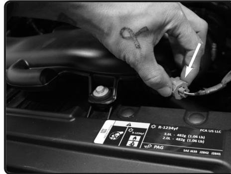
2. Carefully disconnect the temperature sensor, pull back the harness from the intake tube.
