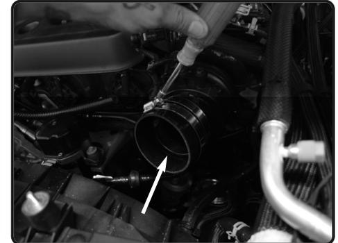
8. Install the provided step hump hose to the throttle body. Secure using provided clamps.
