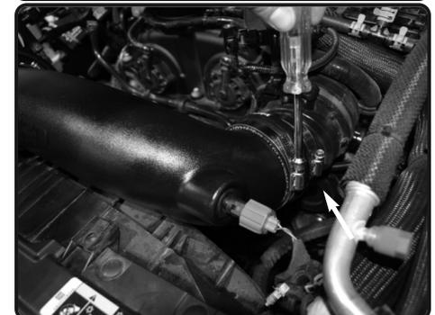
**20.** Secure and tighten all the clamps on the intake tube using 8mm nut driver.
