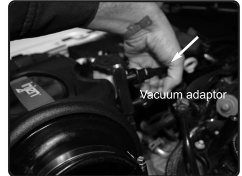
**16.** Connect the vacuum lines to the vacuum adaptor on the airbox.
