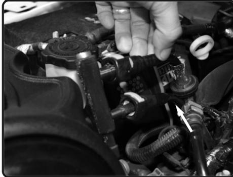
**17.** Make sure the harness on the vacuum lines are secured and you hear the click. Tug and pull back to verify they're connected.
