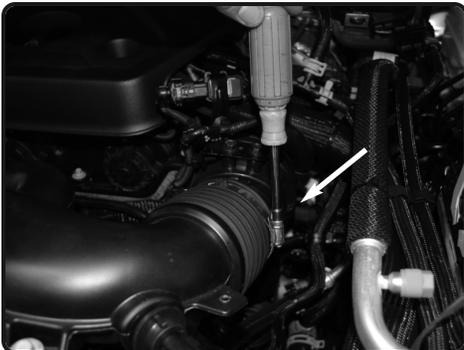
5. Loosen the clamp on the turbo inlet and pull back the intake tube from the turbo inlet.
