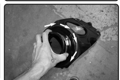
12. Once the twist lock filter is seated properly, rotate the filter in either direction a 1/4" turn until filter locks into place.
