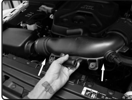
6. Lift up and remove the stock intake system out of the vehicle with air box..
