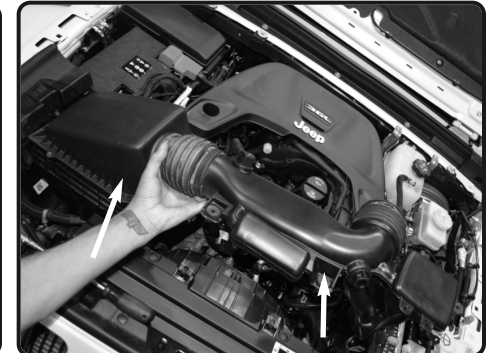
7. Now lift up and remove the air box assembly out of the vehicle.
