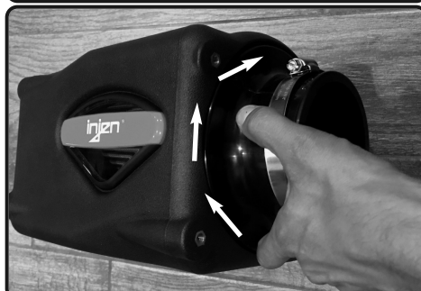
9. 1) Insert twist lock filter to the air box. 2) Once seated, rotate in either direction 1/4 turn till filter locks.
