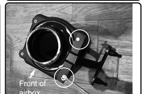
11. Install the provided Bracket to the powerflow box using provided M6 screws. Secure and tighten.
