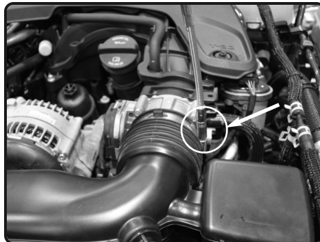
5. Loosen the clamp on the throttle body using 8mm nut driver.
