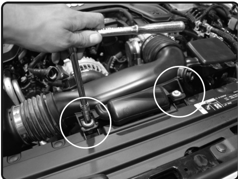
4. Loosen the 2 bolts holding in the intake tube using 10mm socket or ratchet.
