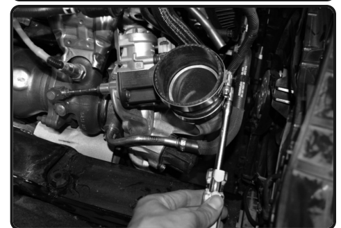
11. Tighten the clamp on turbo only.
