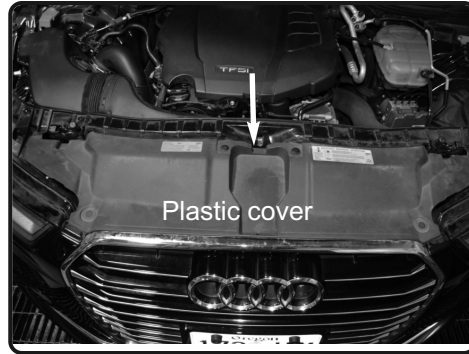
2. Front plastic cover needs to be removed for access to the air box scoop.
