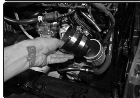
10. Install the provided step hose with clamps provided to turbo.
