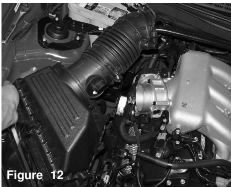
Figure 9 The tension clamp on the crankcase vacuum line is compressed and pulled back, this will allow you to remove the hose from the air duct port.
