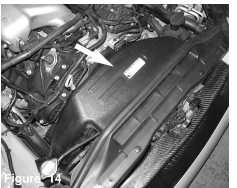
Figure 13 View of the stock air intake box and air intake duct.
