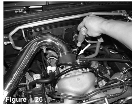
Figure 26 Tighten clamp using 8mm nut driver.
