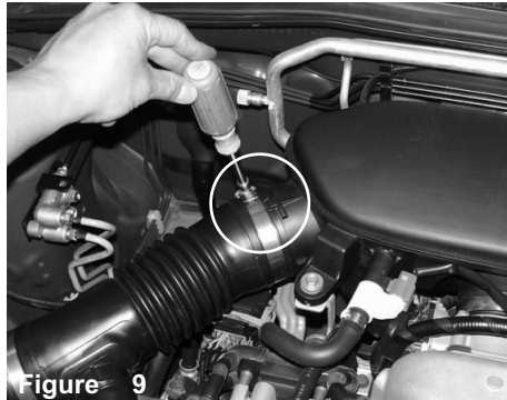
Figure 8 Carefully remove the MAF sensor.
