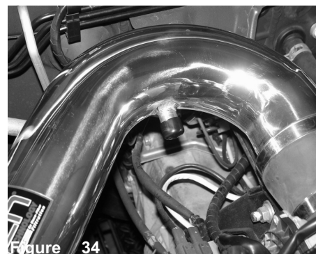
Figure 34 2005 model only cap off the 5/8 fitting.
