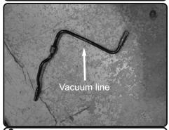
**6.** Vacuum line removed from the vehicle.
