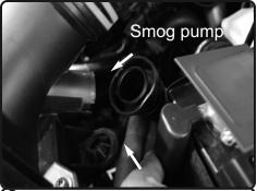
**3.** Disconnect the smog pump line from the stock air box fitting.
