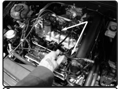
**5.** Pull back the vacuum line from the engine fitting and remove.
