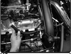
**17.** With provided 10mm vacuum hose, connect the line to the fitting on the intake tube.
