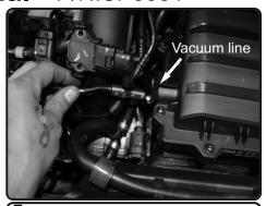
7. Disconnect the vacuum line from the air box.
