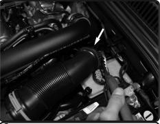
**2.** Loosen the clamp using pliers and pull back the intake tube from the turbo.
