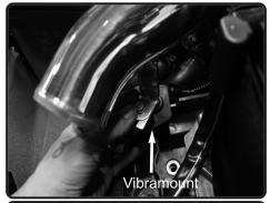
**14.** Secure the bracket using provided M6 nut and fenderwasher and secure.
