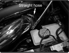
**15.** Position the tube for best fit, secure and tighten the clamps using 8mm nut driver.
