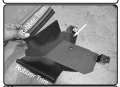
**10.** Install the rubber trims to the top and front of heatshield..
