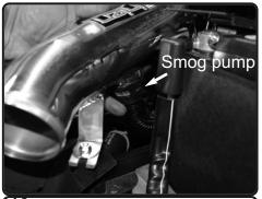
**16.** Reconnect the smog pump line to the fitting on the intake tube.
