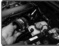
**7.** Install the provided 2.5" straight hose with clamps to the turbo. Tighten the clamp on the turbo only.
