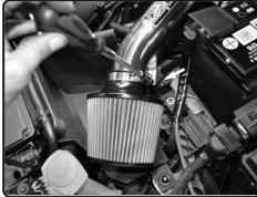
**19.** Install the air filter to the intake tube and tighten using 8mm nut driver.
