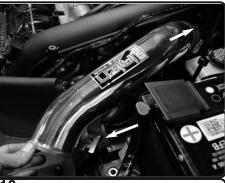
**13.** Install the intake tube and position the intake tube to the turbo and bracket to the vibramount on heatshield.
