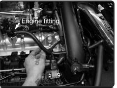
**18.** Now install the 10mm hose to the fitting on the engine. Secure line to desired position.
