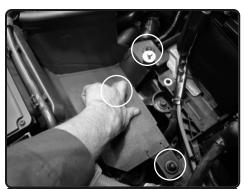
**12.** Make sure the 3 grommets are seated to the factory air box studs in the vehicle.
