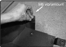
**9.** Install the M6 vibramount to the thredded insert on the heatshield and secure.
