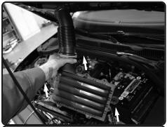
**4.** Pull back the intake tube from the turbo, now lift up and remove the entire intake system out the of vehicle.
