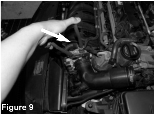
Figure 9 Use a channel lock plier to loosen the pressure clamp on the throttle body and remove the plastic air duct from the throttle body.
