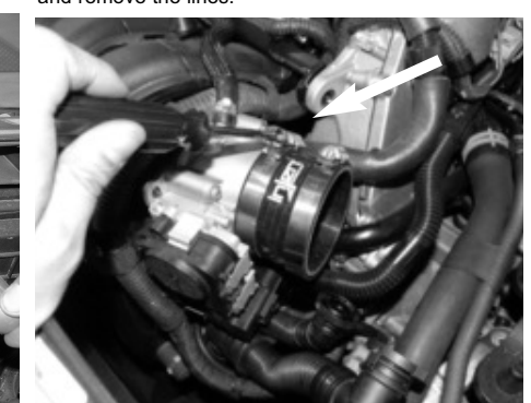
Figure 11 Install the straight hose with clamps to the throttle body. Tighten the clamp on throttle body only using 8mm nut driver.
