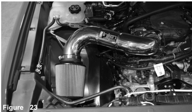
Figure 23 Congratulations! You have just completed the installation of this intake system. Periodically, check the alignment of the intake, normal wear and tear can cause nuts and bolts to come loose. Note: Check clearance and adjust if needed! Failure to check the alignment and adjust the intake can cause damage that will void the warranty. Injen Technology is not responsible for any damages caused by/from improper installation...
