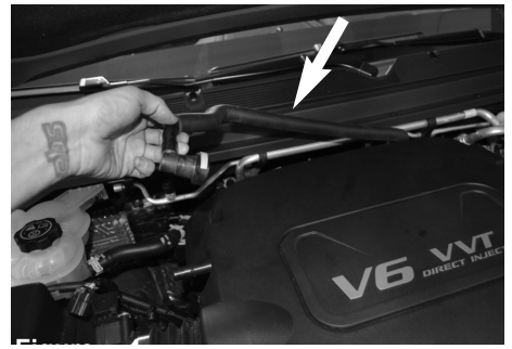
Figure 4 Pull the cranksense line from the back of the engine cover/airbox.
