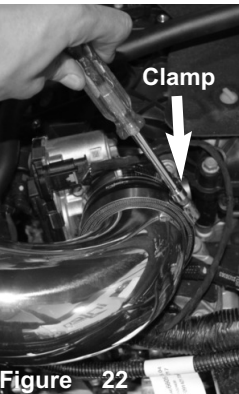
Figure 22 Adjust for the best position and tighten the clamp on the throttle body using 8mm nut driver. Install air filter to the intake tube and tighten using 8mm nut driver.
