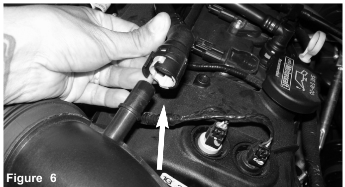
Figure 6 Disconnect crank case line from intake tube.
