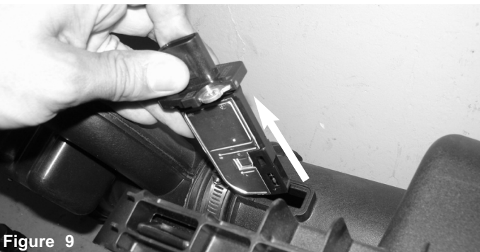
Figure 9 Carefully pull out the MAF sensor and set aside.
