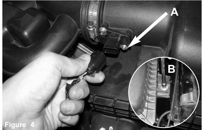
Figure 4 A) Disconnect the MAF sensor from harness. B) Loosen the 10mm bolt holding in the air box.
