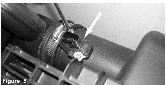
Figure 8 With T25 torx bit, loosen and remove the stock MAF sensor from the air box.
