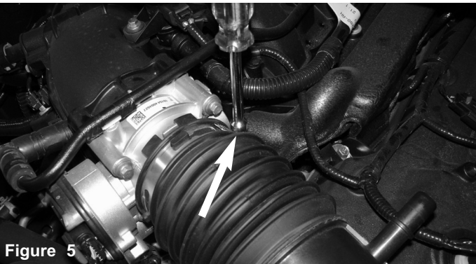
Figure 5 Loosen the clamp on the turbo using 8mm nut driver
