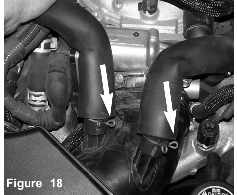
Figure 15 The harness clip is also removed from the vacuum switching valve.
