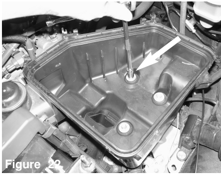
Figure 22 Loosen and remove the 3 bolts holding in the stock bottom half of the air box.
