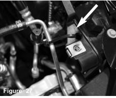
With provided zip-tie, secure the A/C line to the front core support hole. Note: Injen Technology is not responsible or liable for damage to A/C line or intake system and will not be covered under warranty for inproper installation or clearance issues.
