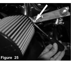
Secure and tighten using 8mm nut driver.
