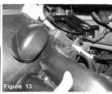
Now remove the resonator scoop from the air box
