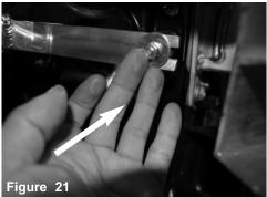
Secure the vibramount with the provided M6 nut and fender washer.
