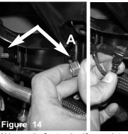
A) Loosen the 2 nuts using 13mm socket or wrench holding in the air box bracket.
