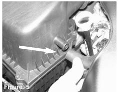
Pull back the crank case line from the air box.
