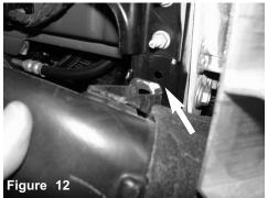
Remove the clips holding in the resonator scoop on vehicle frame.
