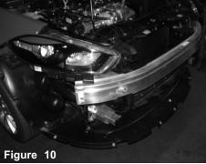
Remove the front bumper cover. Loosen and remove clips and screws on top, side and bottom of cover. Carefully remove the cover.
