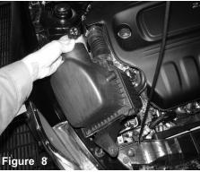
Pull out the air box assembly from the vehicle.
