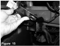
Remove the air box bracket.
