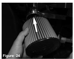
Install the filter to the tube.
