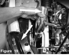
Install the intake tube into the vehicle. Position the bracket to the vibramount. Position the upper part of the tube to the factory intake hose.
