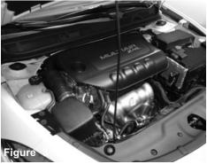
Stock box shown in this picture. Disconnect negative battery terminal.
