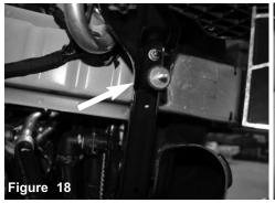
Secure and tighten the vibramount to the vehicle.
