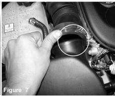
Loosen the clamp on the air box using 8mm nut driver, loosen and pull back.
