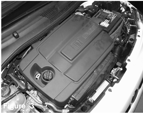
Figure 4 Lift up the engine cover, and remove.
